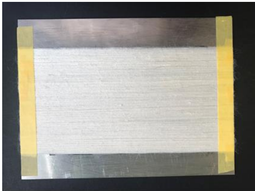
Fig. 1. Completed prepreg of ramie yarn
