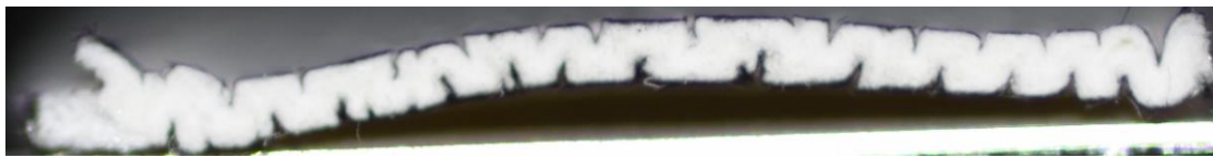
Fig. 10. Paperboard sample after the IPCTM from the test series depicted in Fig. 9, with distinctive wrinkle formation
