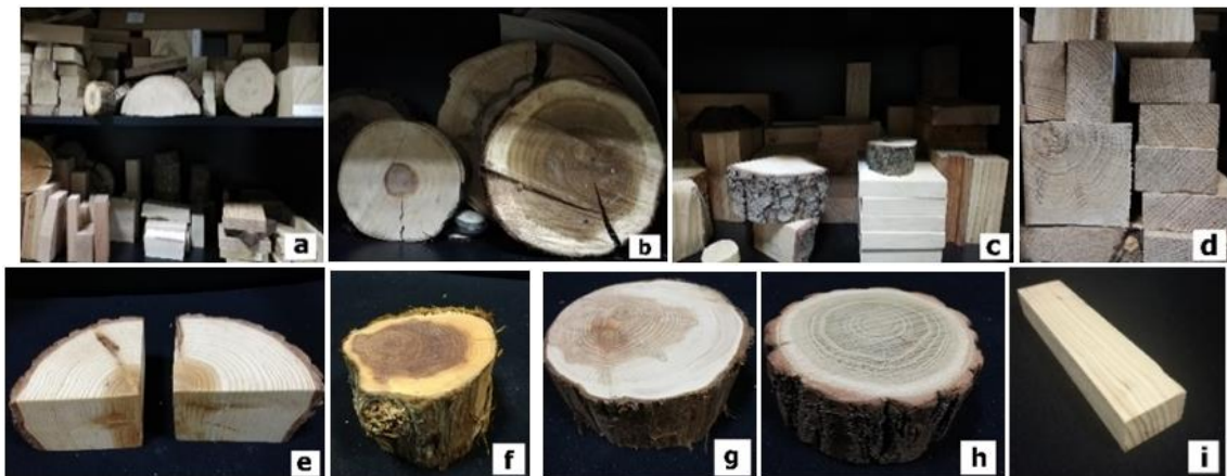
Fig. 3. Some wood samples used in the classroom: (a-b-c-d) wood from the author's collection, (e) softwood sections, (f)-(g) juniper ( Juniperus sp.), (h) black locust ( Robinia pseudoacacia ), (i) fir ( Abies sp.).
