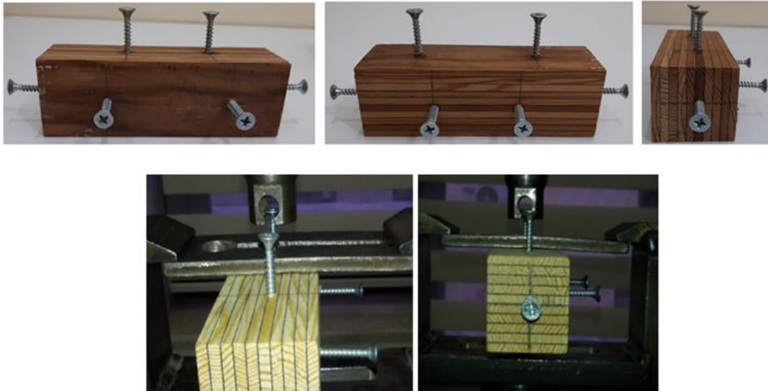
Fig. 3. Test samples and setup used for the screw withdrawal tests
