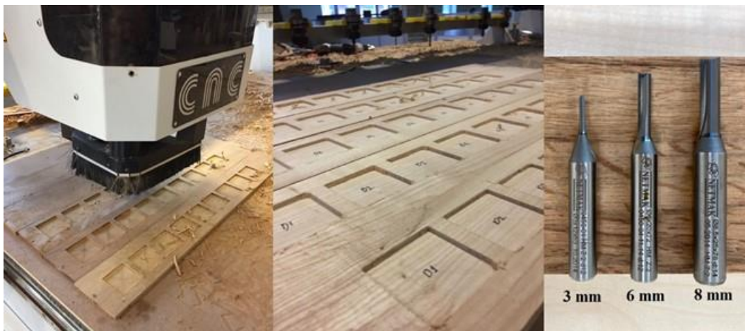
Fig. 1. CNC processing of wood samples and the used cutting tools
