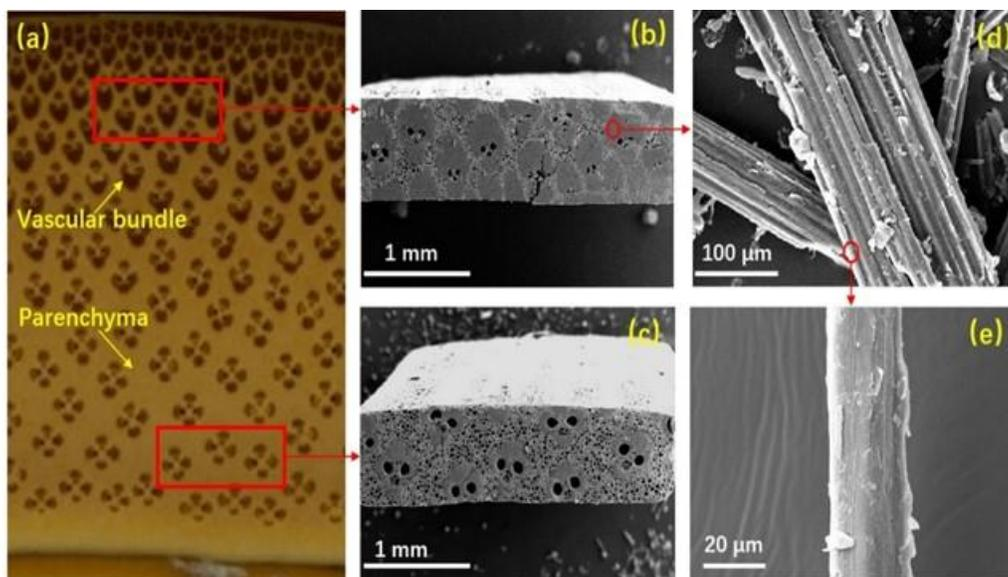
**Fig. 1.** The structure of the bamboo units at multi-scale: (a) bamboo culm; (b) a sliver from the outer bamboo; (c) a sliver from the inner bamboo; (d) a bamboo fiber bundle; and (e) an individual bamboo fiber
