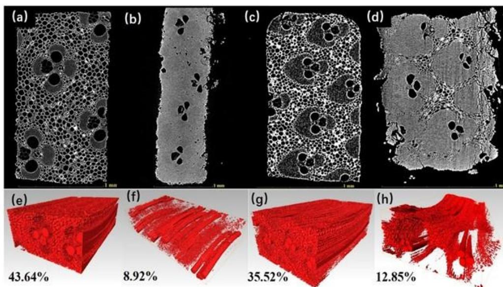
**Fig. 5.** The cross-sectional morphology and pore structure of the bamboo slivers: (a) and (e) the untreated inner bamboo; (b) and (f) the 15% NaOH treated inner bamboo; (c) and (g) the untreated outer bamboo; and (d) and (h) the 15% NaOH treated outer bamboo
