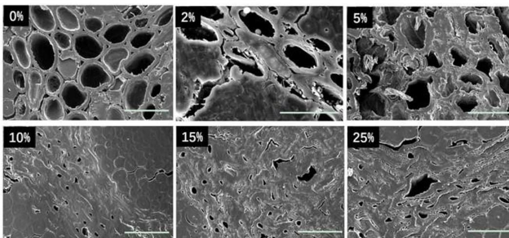
**Fig. 4.** Cross-section of parenchyma cells in the slivers from the outer layer of the bamboo treated with different concentrations (scale bar = 50  $\mu\text{m}$ )
