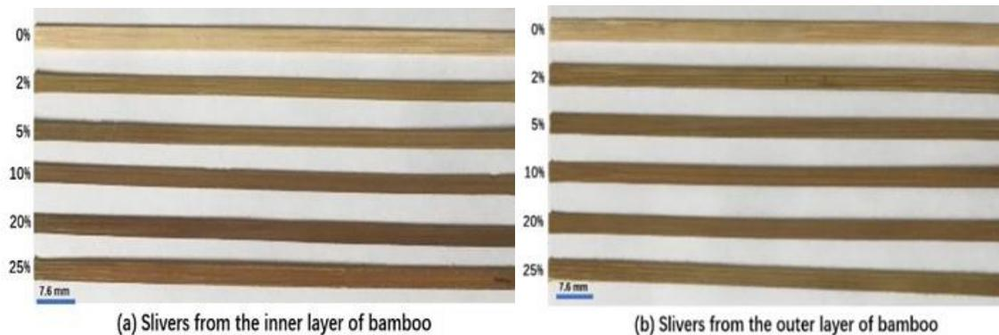
**Fig. 2.** Photographs of the untreated and treated bamboo slivers showing the change in the color: (a) the inner layer; and (b) the outer layer
