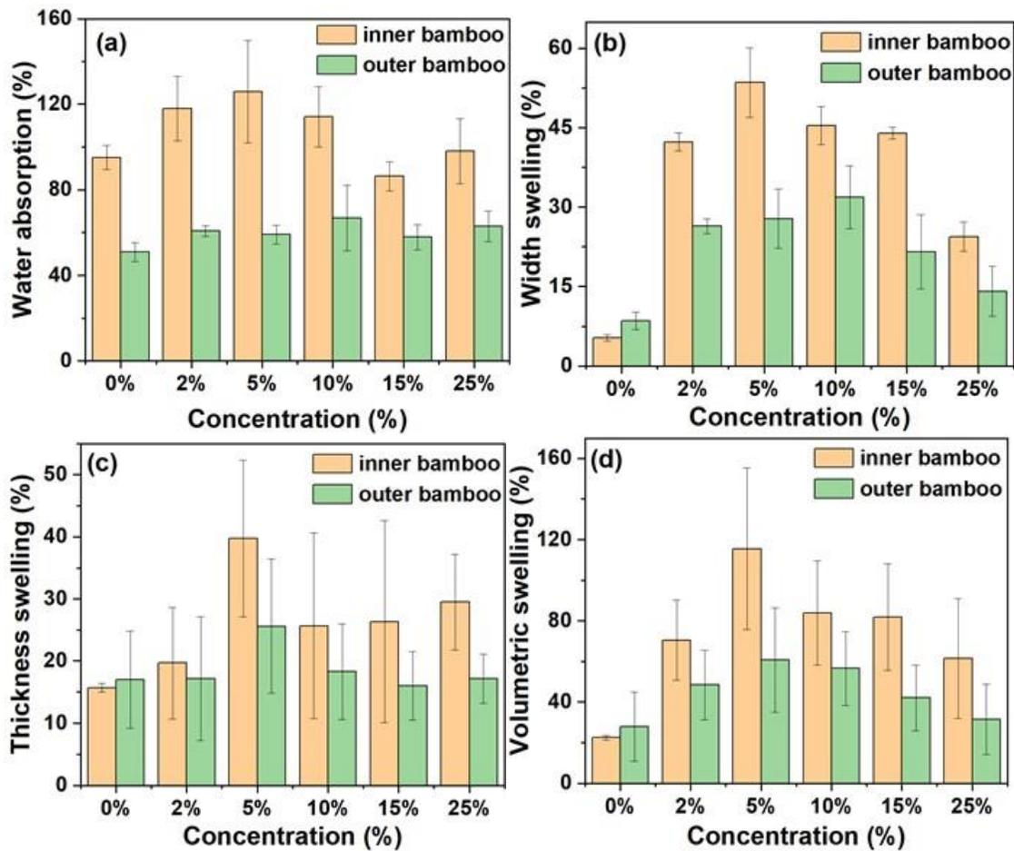
**Fig. 6.** The water absorption and dimensional stability of the bamboo slivers: (a) water absorption; (b) width swelling; (c) thickness swelling; and (d) volumetric swelling
