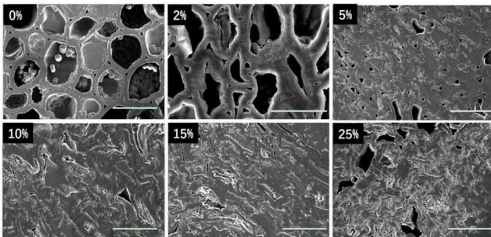
**Fig. 3.** Cross-section of the parenchyma cells in the slivers from the inner layer of the bamboo treated with different concentrations (scale bar = 50  $\mu\text{m}$ )
