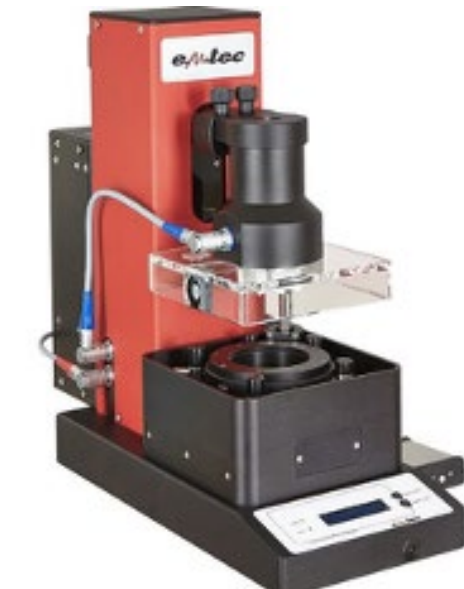
Fig. 4. Emtec's TSA softness measurement device (Paper Technology International 2021)
