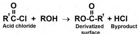
Scheme 9. Reaction of an acid chloride with an –OH group of a polysaccharide-based substrate
