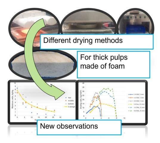
A graphical abstract that summarizes research on drying methods involving thick foam mats. Timofeev, O. N., Jetsu, P., and Keranen, J. T. (2022). "**Drying of thick foam formed mats comprising chemithermomechanical pulp fibers**," *BioResources* 17(2), 2547-2562.
