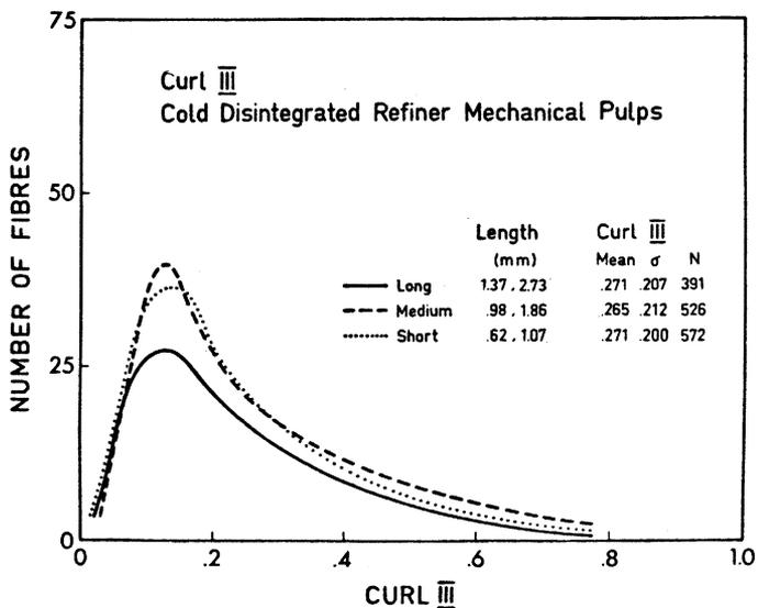
Fig 12—The Curl III distributions for three length classifications of the cold disintegrated refiner mechanical pulp.
