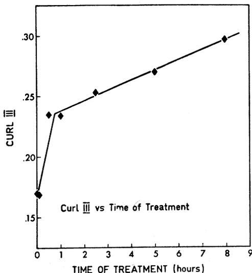
A commercial predominantly spruce, kraft pulp was beaten to 1000 Rev. in a PFI mill and then subjected to curling at 20% consistency in a Hobart kitchen mixer. After various times of treatment, samples were withdrawn and prepared for image analysis. Figure 9 shows the change in Curl III with time of treatment. We see that the curl increases dramatically in the first half hour and then
