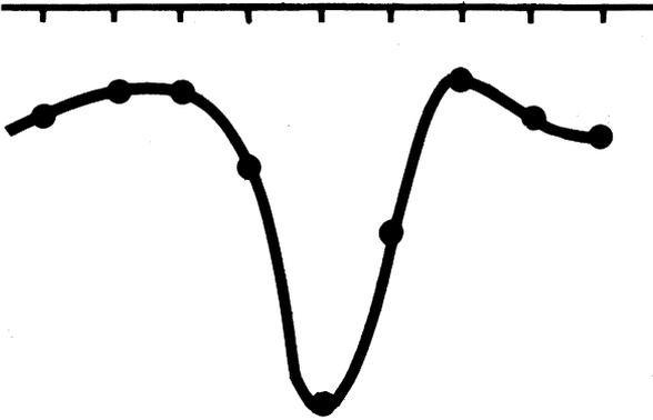
The question that then arises is whether any one pixel forms part of the fibre image or not. We look at the intensity values of the individual cells and fit a curve through these points. If we know the response function of the microscope then a proper measurement of width can be derived though the arguments are complex.
