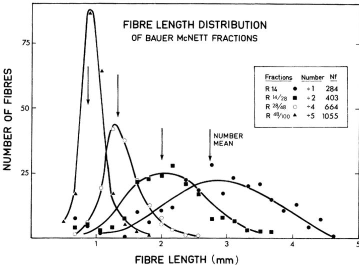
**Fig 3**—The fibre length distributions for four Bauer McNett fractions. The arithmetic mean (as opposed to the weighted mean) is indicated by the arrows. The legend indicates the total number of fibres in the sample ( $N_f$ ) and the scale factor.
