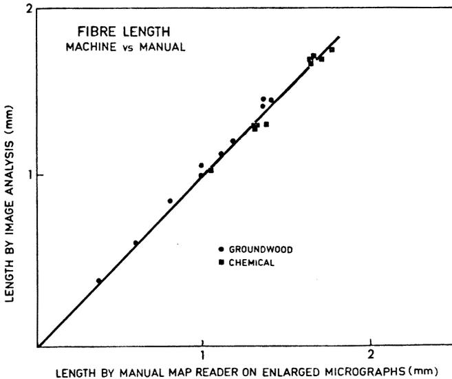
Fig 2—Comparison of the length of some chemical and mechanical pulp fibres measured by image analysis and by manual procedures.
