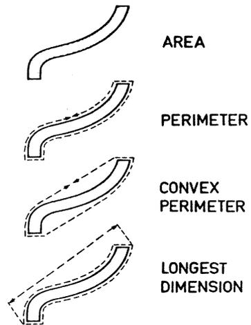
Fig 1—Four of the basic measurements that can be made using the fast logic circuitry.
