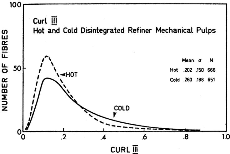
Fig 11—The Curl III distributions of a hot and a cold disintegrated refiner mechanical pulp.
