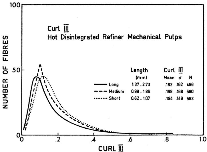
Fig 13—The Curl III distributions for three length classifications of the hot disintegrated refiner mechanical pulp.
