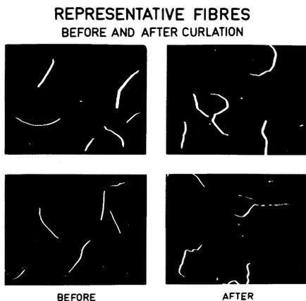
Fig 6—Fibres before and after curlation, photographed from the screen of the image analyzer.
