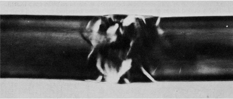
**Fig 5**—Node in laboratory softwood kraft pulp, unbeaten (X1,000).
