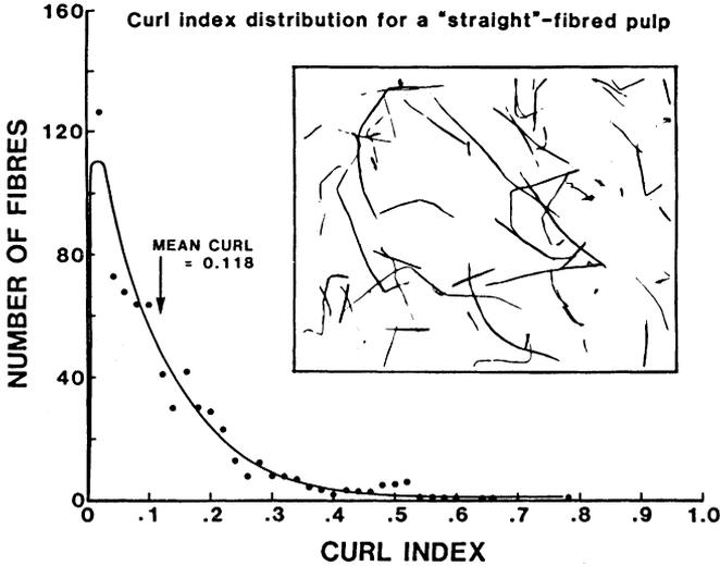
**Fig 10**—Typical curl index histogram of a straight-fibred pulp, inset with a micrograph of the fibres. The measurements were made on a sparser deposition of the same fibre population as that shown here. the pulp is a softwood high-yield sulphite.
