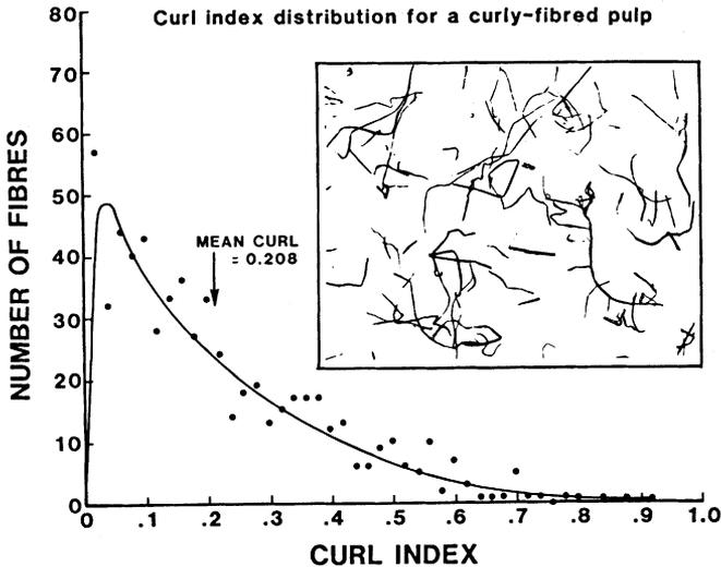
**Fig 11**—Typical curl index histogram of a curly pulp. This is the same high-yield sulphite pulp as in the previous figure, but curl-set by steaming for 5 min. at 160°C. Many of the fibres are still straight, but an increased fraction of the fibres have become quite curly.
