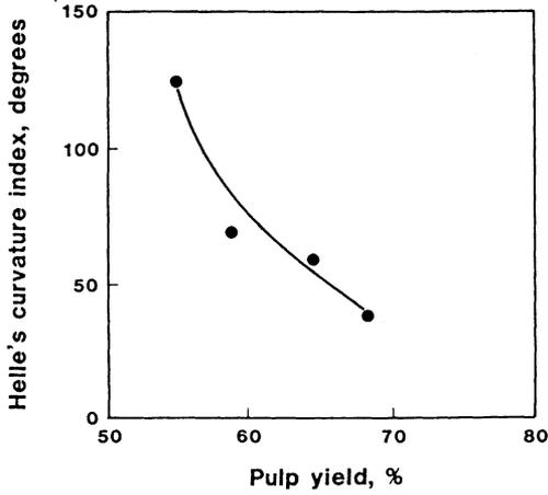
**Fig 12**—Data of Helle (16) showing the effect of pulp yield on curvature index for sulphite pulp fibres which had been given a mild mechanical treatment at high consistency.
