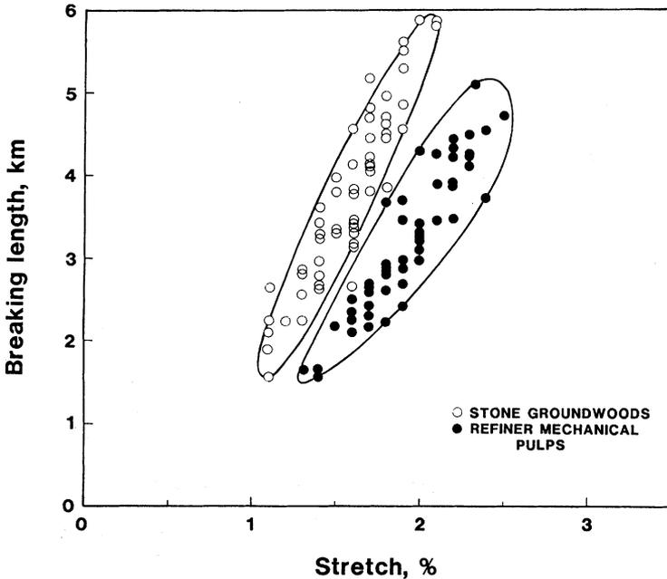
Fig 17—Breaking length against stretch for handsheets of laboratory mechanical pulps. At a given tensile strength the refiner mechanical pulps, which contain microcompressions, have a higher stretch, as shown by Page and Seth (60). Data of de Montmorency (61).
