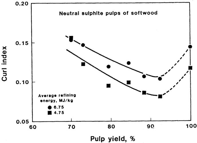
**Fig 13**—Plot of curl index against pulp yield for neutral sulphite pulps. the curl indices are compared at constant input of refining energy. The pulps were refined in a double-disc refiner at about 20% consistency.
