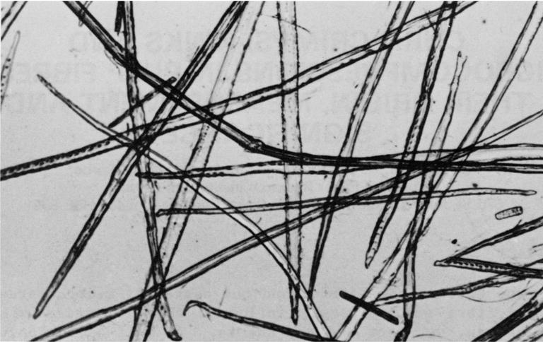
**Fig 1**—Straight fibres of commercial softwood bisulphite pulp of 62% yield (X60).
