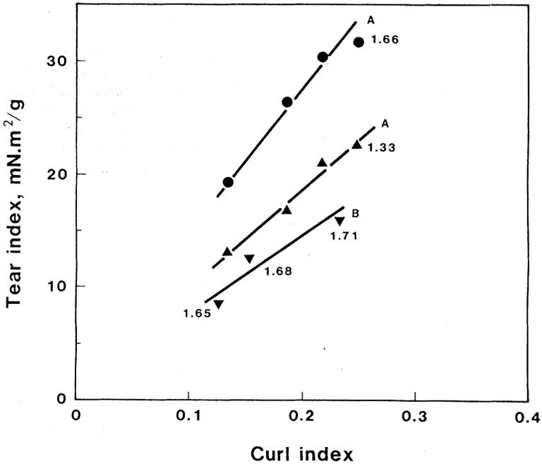
Fig 16—Plot showing the effect of fibre curl on dry-sheet tear index. The numbers against lines and data points indicate sheet bulks in cm<sup>3</sup>/g. Experiments A and B correspond to those in Figure 15.
