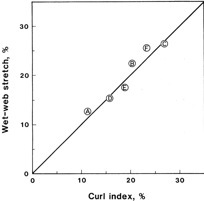
**Fig 14**—Plot showing the excellent correspondence between wet-web stretch at low solids and fibre curl index, expressed as a percentage, for very conformable fibres. A and B — thermomechanical pulps of softwood, original and curl-set, followed by delignification with acidified sodium chlorite. C — commercial dried unbleached softwood kraft pulp, beaten and then curled at high consistency. D, E and F — 46% — yield unbleached softwood sulphite pulp, curled and refined at low consistency.
