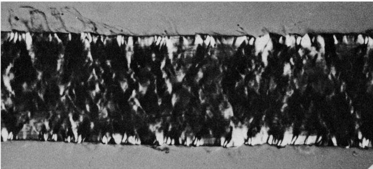
**Fig 7**—Microcompressions in commercial dried bleached sulphite pulp (X600).
