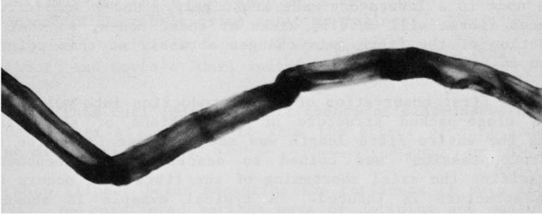
**Fig 6**—Kinks at nodes in commercial dried bleached sulphite pulp (X250).
