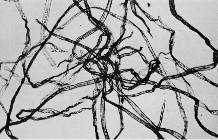
**Fig 3**—Highly curled fibres of commercial flash-dried bleached softwood kraft pulp (X60).
