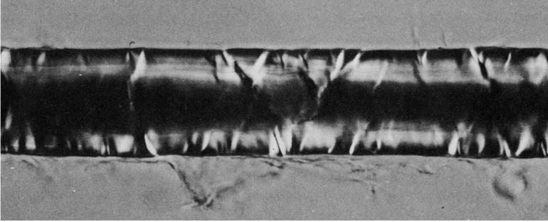
**Fig 4**—Dislocations and slip planes in commercial dried unbleached softwood kraft pulp (X600).
