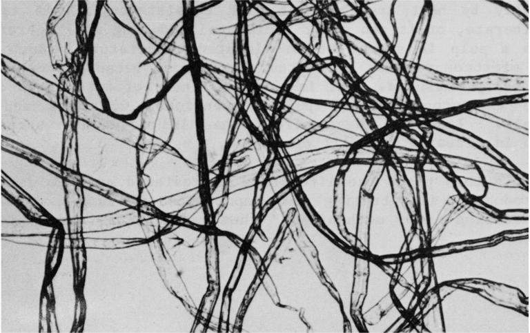
**Fig 2**—Moderately curly fibres of commercial dried bleached softwood kraft pulp (X60)
