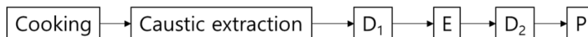
Fig. 3. Bleaching with caustic extraction; D, E, and P stand for chlorine dioxide, alkaline extraction, and hydrogen peroxide, respectively
