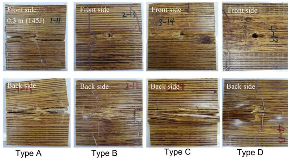
**Fig. 6.** Representative photos of the damage progression on the front and back sides of the four types of bamboo bundle composite panels impacted at 0.3 m (approximately 145 J)
