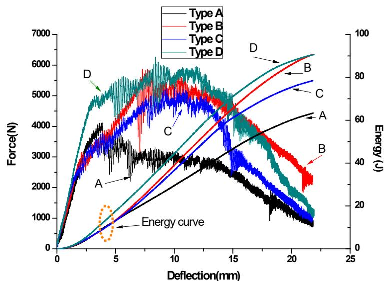
**Fig. 8.** The typical force vs. the displacement response for the 0.2 m test (approximately 95 J) impact response on the four types of bamboo bundle-based composites
