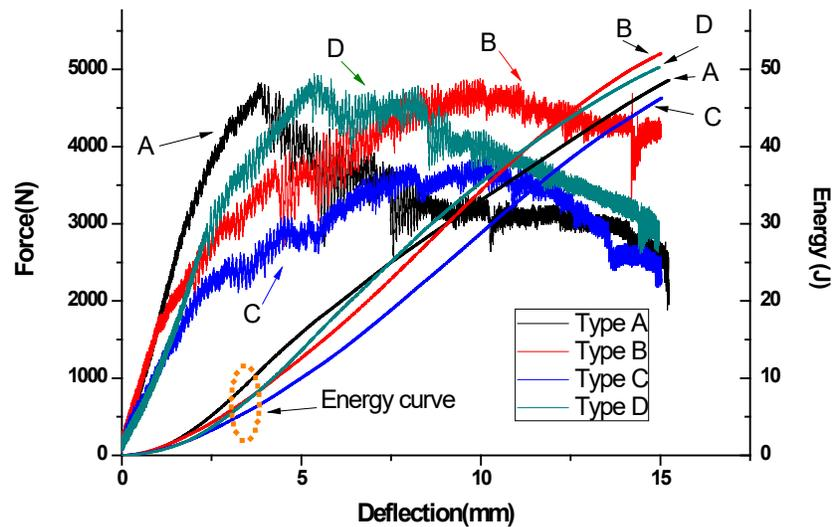
**Fig. 7.** The typical force vs. the displacement response for the 0.1 m test (approximately 50 J) impact response on the four types of bamboo bundle-based composites
