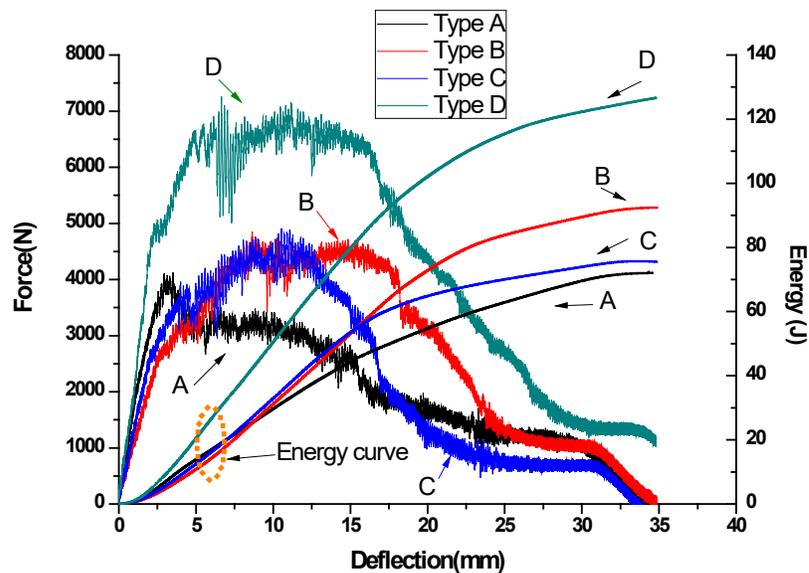
**Fig. 9.** The typical force vs. the displacement response for the 0.3 m test (approximately 145 J) impact response on the four types of bamboo bundle-based composites
