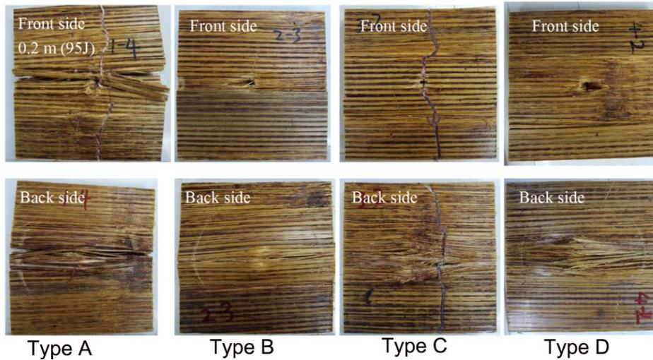
**Fig. 5.** Representative photos of the damage progression on the front and back sides of the four types of bamboo bundle composite panels impacted at 0.2 m (approximately 95 J)
