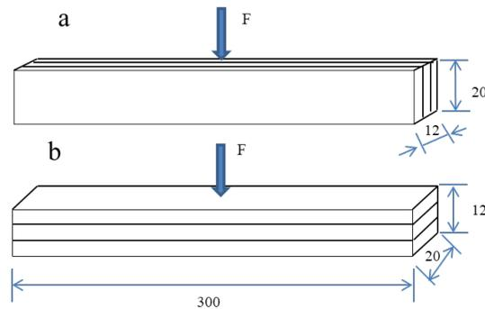
**Fig. 3.** Schematic of two loading directions (The direction of a is parallel to glue line, b is perpendicular to glue line.)
