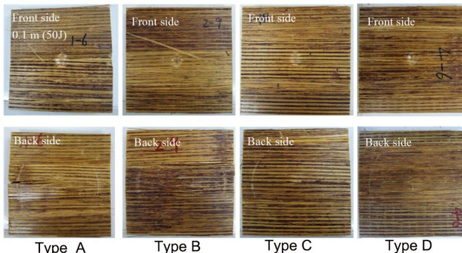
**Fig. 4.** Representative photos of damage progression on the front and back sides of the four types of bamboo bundle composite panels impacted at 0.1 m (approximately 50 J)
