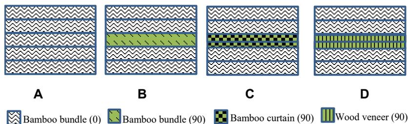
Fig. 2. The schematic illustrations of the bamboo/wood sheet laminate composites
