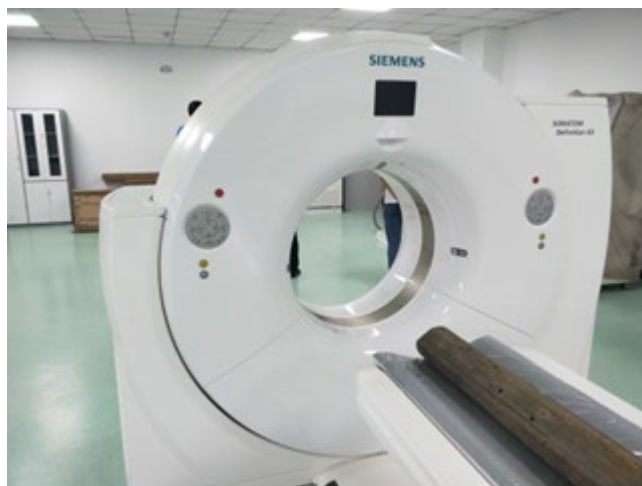
Fig. 2. X-ray CT used to investigate the timber in Shandong Jianzhu University, China
