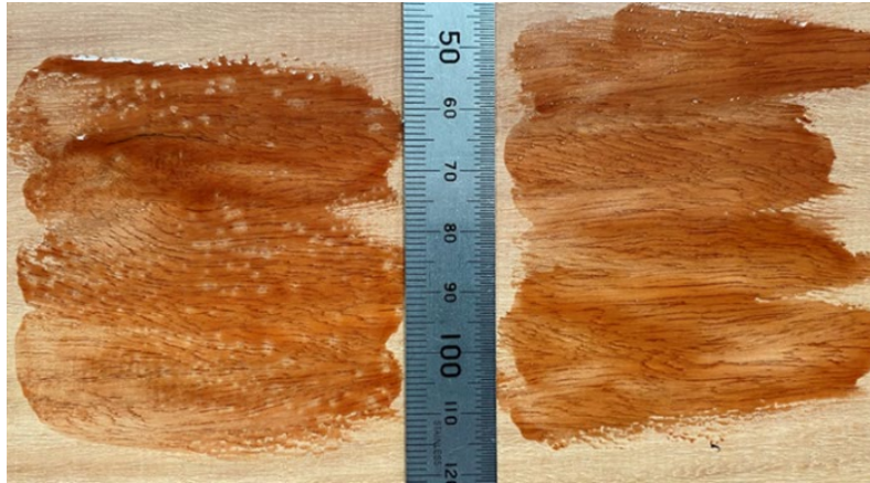
Fig. 4. Resorcinol formaldehyde adhesive application to spotted gum timber without the added surfactant (left) and with the added surfactant (right)
