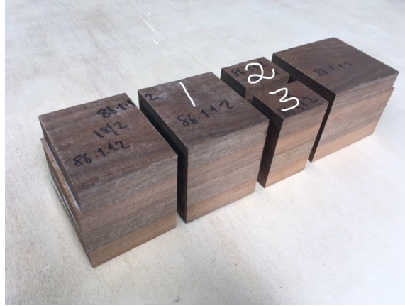
Fig. 2. Post-cure processing of the cured glulam sample: (1) 84 mm x 88 mm x 75 mm (W x T x L) sample for the delamination testing in accordance with AS/NZS standard 1328.1:1998 (2011); (2) 40 mm x 88 mm x 53 mm (W x T x L) sample for block shear testing pre-wet and dry cycling; and (3) 40 mm x 88 mm x 53 mm (W x T x L) sample for fibre failure testing post-wet and dry cycling
