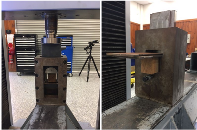
Fig. 3. Block shear testing apparatus
