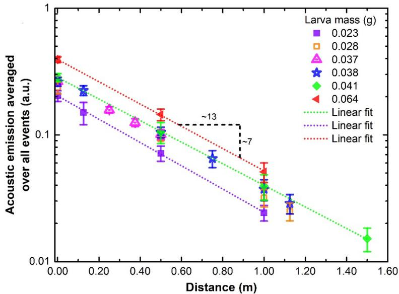
**Fig. 2.** Dependence between calculated acoustic energy of carving wood larvae and the sensor distance in the elements with dimension of  $5.5 \times 11.0 \times 203$  cm; the average standard deviation for each point is marked.
