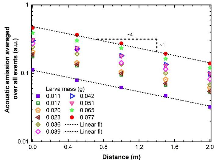
**Fig. 3.** Dependence between calculated acoustic energy of carving wood larvae and the sensor distance in the strips with dimensions of  $1.5 \times 1.5 \times 203$  cm; the average standard deviation was omitted to make the graph more readable. The obtained values of the average standard deviation are comparable with those presented in Fig. 2.
