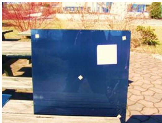
Fig. 3. Starch palmitate (DS 1.5) containing photoactive dye laminated glass possessing photochromic properties (blue - under irradiation with UV light)
