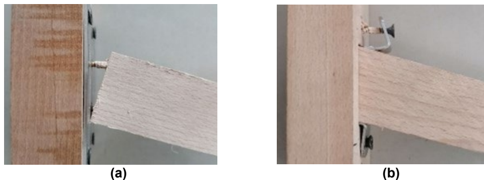
Fig. 7. The failure mode of the experimental a) typical joint and b) novel joint
