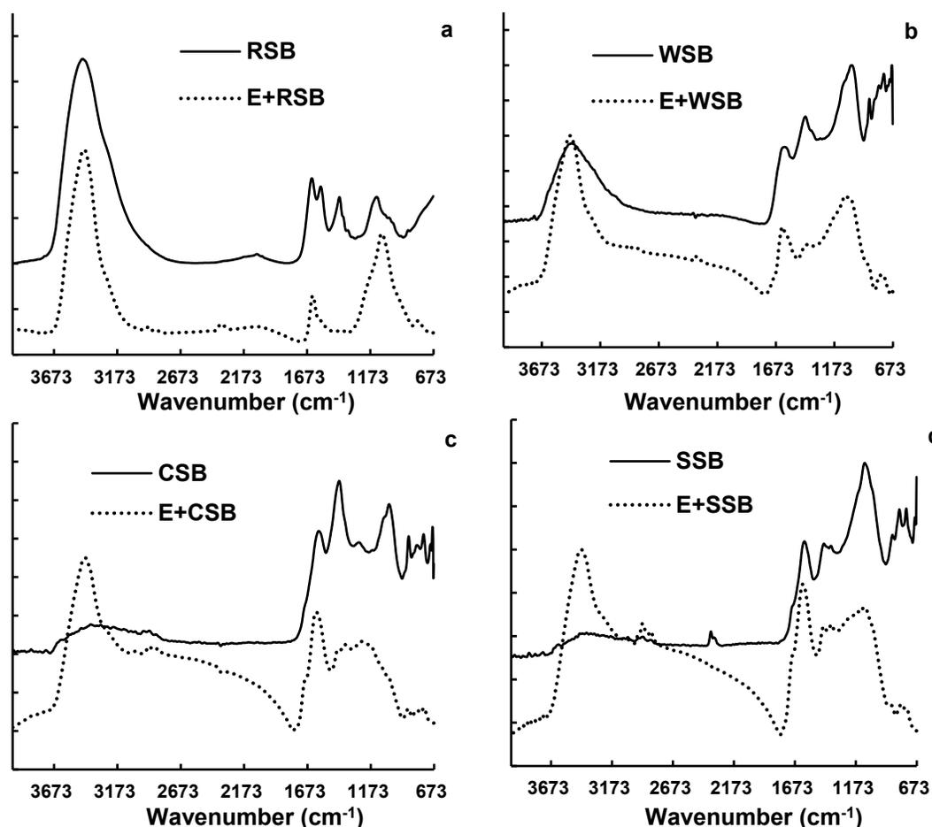
**Fig. 4.** The changes in the fresh and extracted (E+) biochar functional groups (Note: RSB = rice straw biochar (a), WSB = wheat straw biochar (b), CSB = cotton straw biochar (c), SSB = *Spartina alterniflora* biochar (d))
