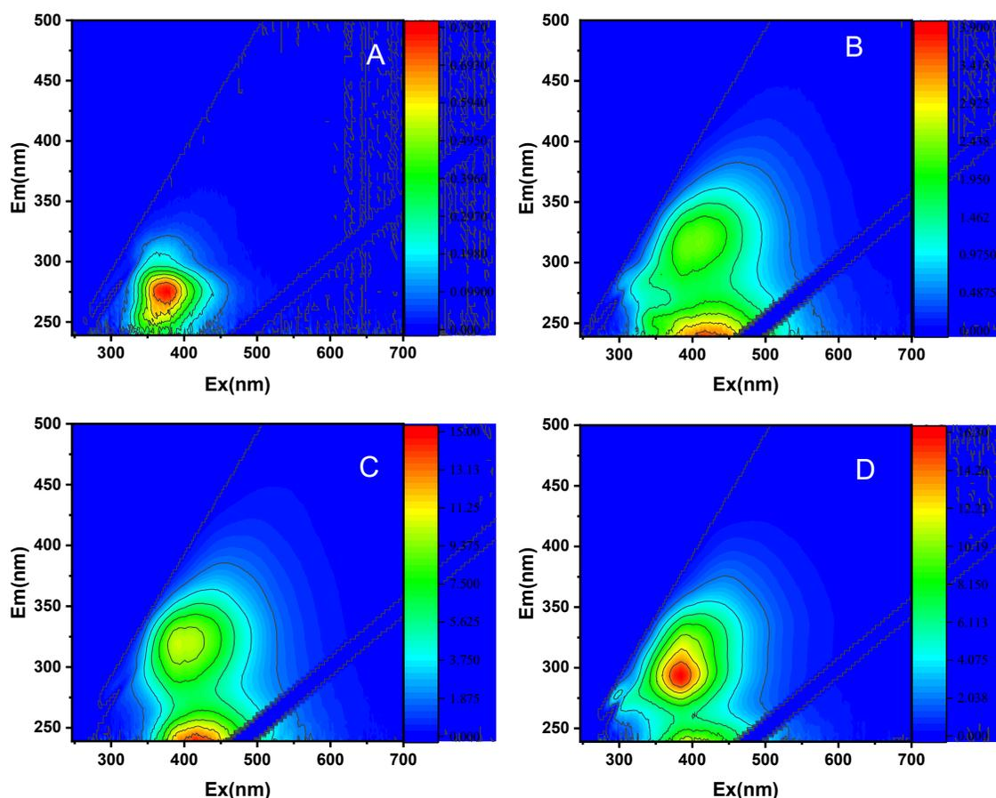
**Fig. 2.** Three-dimensional fluorescence spectrum of the water-soluble organic matter in the biochar extract solution (A: RSB, rice straw biochar; B: WSB, wheat straw biochar; C: CSB, cotton straw biochar; D: SSB, *Spartina alterniflora* biochar)
