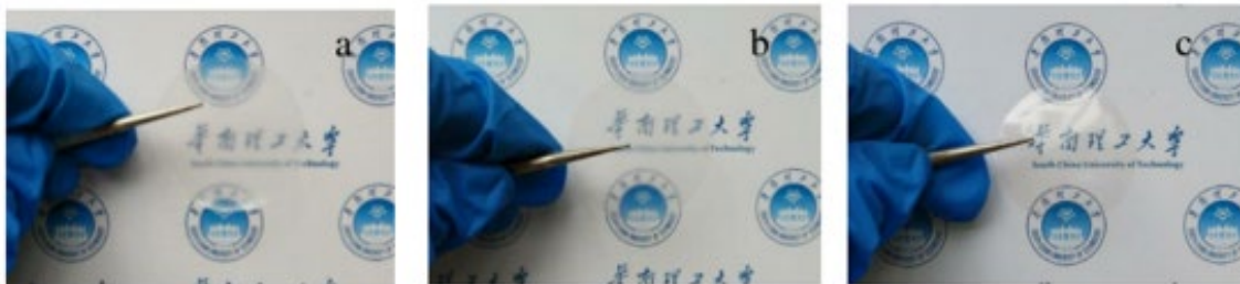
Fig. 7. Digital images of starch (a), NFC/starch(b) and NFC/starch/ nanoparticles (c) films
