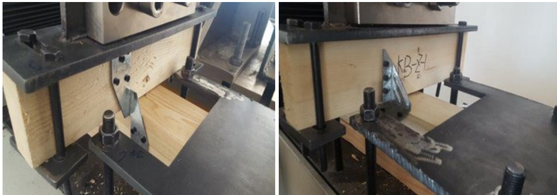
Fig. 2. The fixing method of specimen on equipment (TA-Group and TB-Group)
