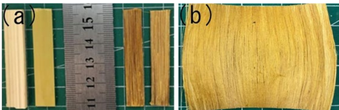
Fig. 1. Processing of bamboo fibers: (a) culms cut to pieces before and after alkali treatment from left-side; (b) a bamboo sheet after hot-pressing
