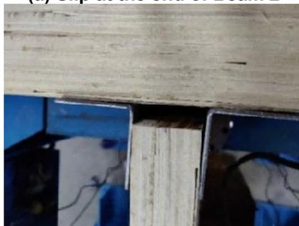
**(c)** Separation between the end of Beam B-2 and the side beam
