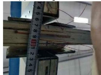
**(d)** Pull-out of the self-tapping screws at the connection
