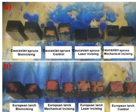
**Fig. 5.** Using chrome azurol-S reagent to detect Cu uptake levels in a) Caucasian spruce and b) European larch wood samples. The blue colors show positive responses.
