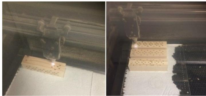
**Fig. 4.** The incision of wood samples by a CO<sub>2</sub> laser
