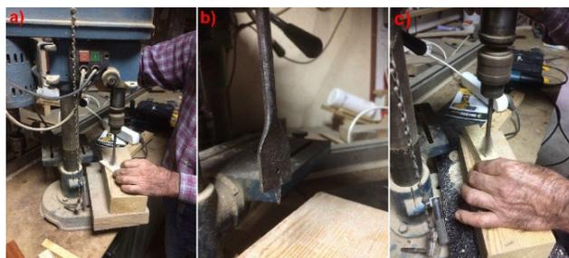
**Fig. 3.** Images depicting the a) preparation of a wood surface die (10,000 incision/m<sup>2</sup>) for all mechanical incising operations, b) the depth of the spade drill bit (10 mm), and c) the incision of wood samples by the spade drill bit
