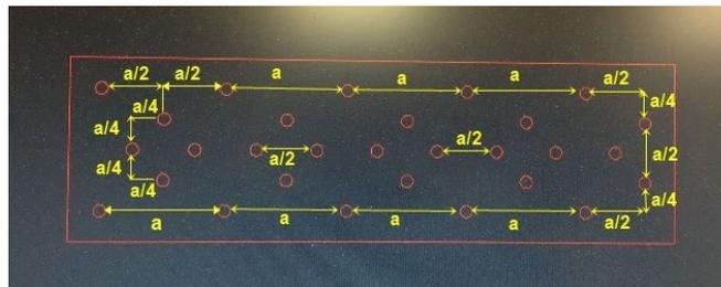
**Fig. 2.** Mechanical and laser incising patterns on radial and tangential surfaces and distances between holes in transverse and longitudinal directions
