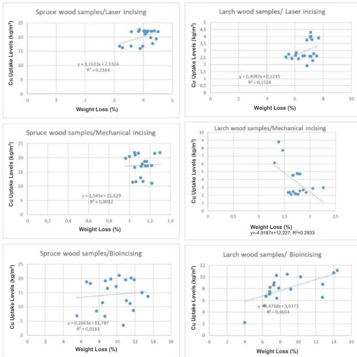
**Fig. 6.** Correlation between the weight losses and Cu uptake levels in the impregnated spruce and larch wood samples pre-incised with the three different incising methods
