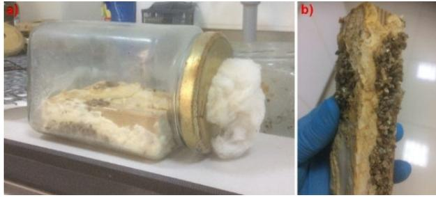
**Fig. 1.** Images of the a) heterogeneous and b) homogeneous colonization of wood samples by *P. vitreus* fungus in glass jars
