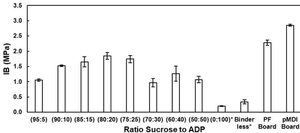
Fig. 2. The IB properties of the particleboards with various ratios of sucrose-ADP (\*Adapted from Komariah *et al.* 2019)
