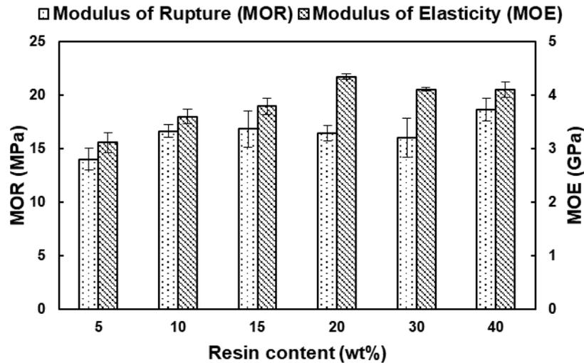
**Fig. 6.** MOR and MOE values of the particleboards with sucrose-ADP 80:20 with various resin contents (wt%)
