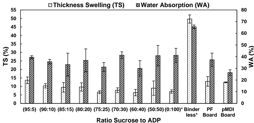
**Fig. 3.** TS and WA values of the particleboards with various ratios of sucrose-ADP (\*Adapted from Komariah *et al.* 2019)
