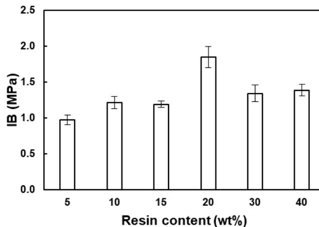
**Fig. 7.** IB values of the particleboards with sucrose-ADP 80:20 with various resin contents (wt.%)
