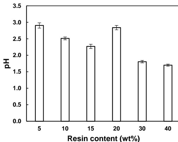
**Fig. 9.** pH of the soaking water after the TS treatment of the particleboards with sucrose-ADP 80:20 with various resin contents (wt%)
