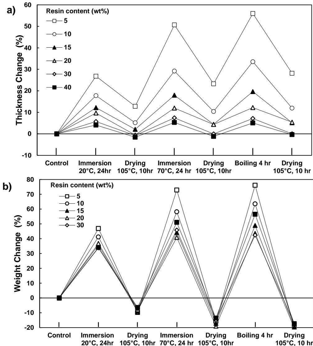
**Fig. 10.** The a) thickness and b) weight changes of the 80:20 sucrose-ADP particleboards with various resin contents (wt%) on the cyclic aging treatment test
