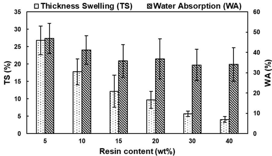
**Fig. 8.** The TS and WA properties of the particleboards with sucrose-ADP 80:20 with various resin contents (wt%)
