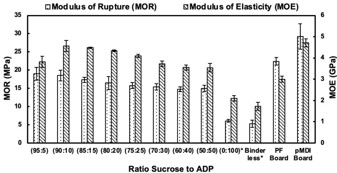
Fig. 1. The bending properties of the particleboards with various ratios of sucrose-ADP (\*Adapted from Komariah *et al.* 2019)
