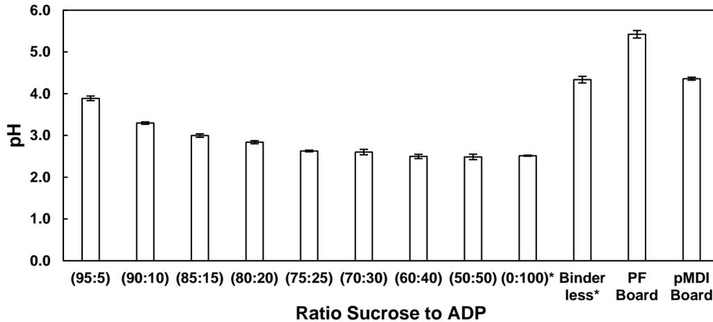
Fig. 4. pH of the soaking water after TS treatment of the particleboards with various ratios of sucrose-ADP (\*Adapted from Komariah *et al.* 2019)
