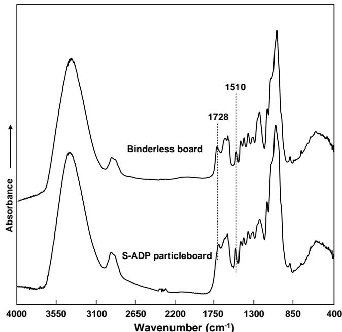
**Fig. 11.** FTIR spectra of the OPT binderless particleboard and the sucrose-ADP particleboard (80:20, resin content of 20 wt%) after the cyclic aging treatment test
