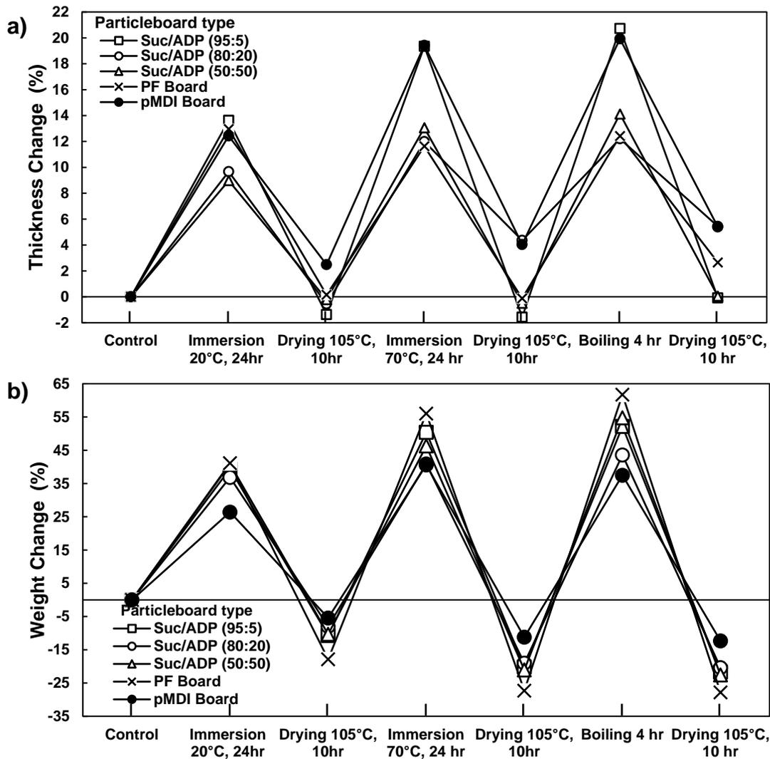
Fig. 5. The a) thickness and b) weight changes of the particleboards with various ratios of sucrose-ADP on the cyclic aging treatment test
