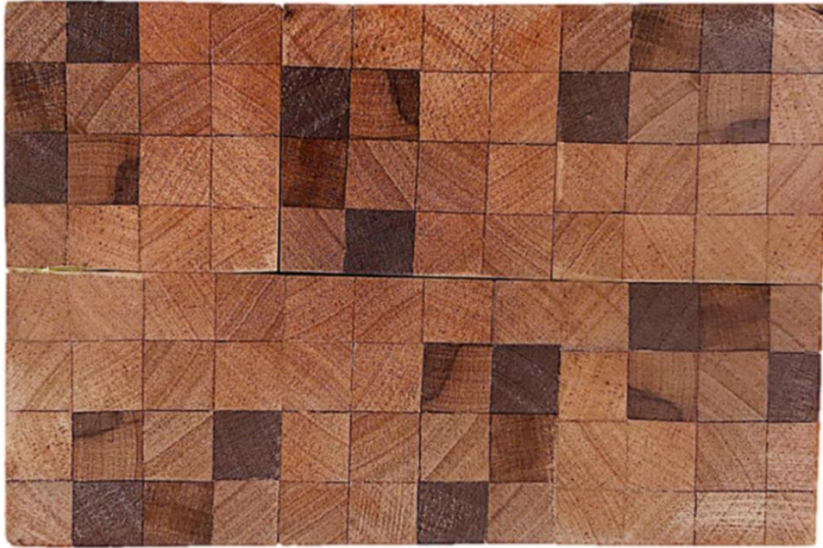
Fig. 4. Sound-absorbing board of Homalium foetidum transverse plane (manufactured by authors)
