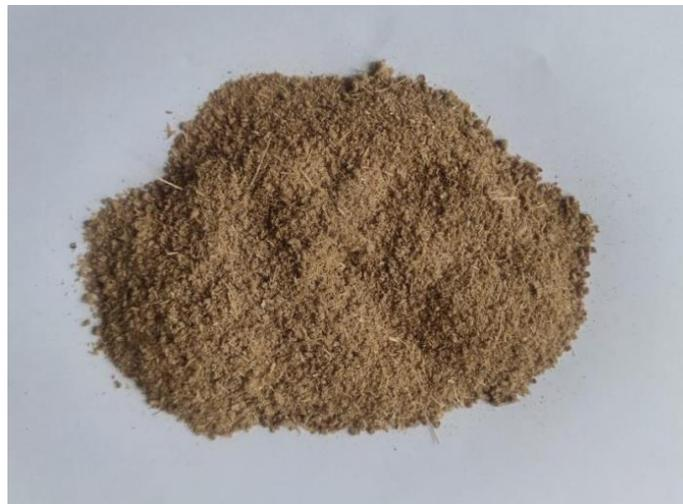
**Fig. 1.** The mixture of cornstalk particle and potato residue
