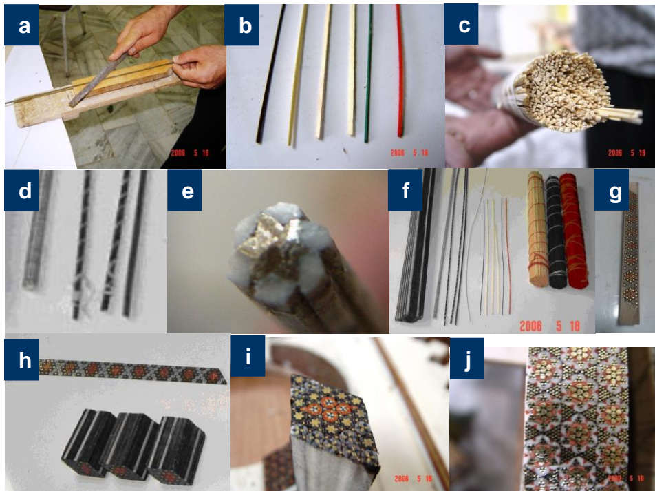
Fig. 2. Grinding triangles inside a triangular mold (a); wood with color and triangular section (b); triangular wood bundle (c); "Pareh" and "Shesh" (d); view of the cross-section of an Ostokhani "Shesh" (e); triangular wood and brass wire, "Pareh", "Shesh", and "Luz" of inlay (f); Qameh (g); 6 cm cut "Luz", and "Barg" of inlay (h); view of cross-section of an "Abri" inlay "Luz" (i); a sample of Haft Shamseh Alam-Zar inlay (j)
