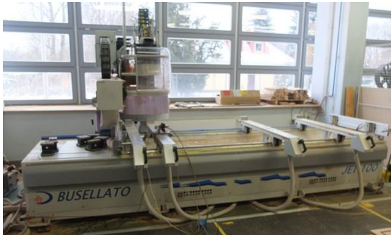
Fig. 4. Busellato JET 100 standard CNC machining center
