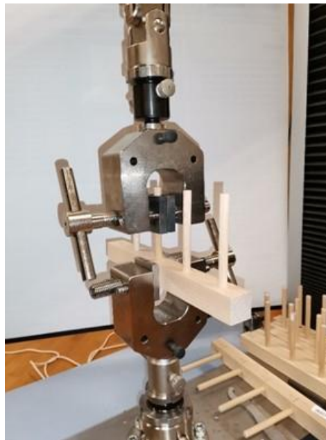
Fig. 3. Positioning of samples during the embedded force testing
