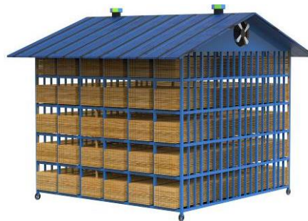
Fig. 10. Bamboo strips storage facility
