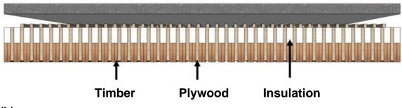
(b) NLT-concrete composite slab
