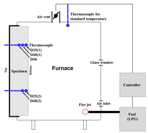
b) Schematic diagram of the furnace-burner system
