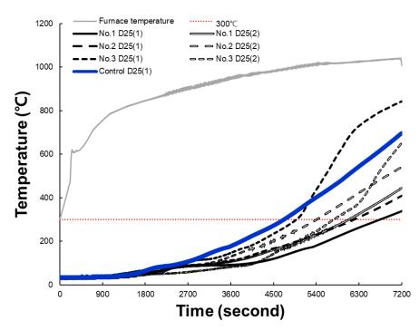
(a) D25 (25 mm depth from the fire exposed surface)
