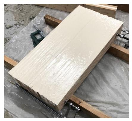
Fig. 3. Intumescent coating on plywood laminae
