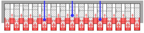
(b) Three-dimensional heat transfer into timber (uncoated specimen)
