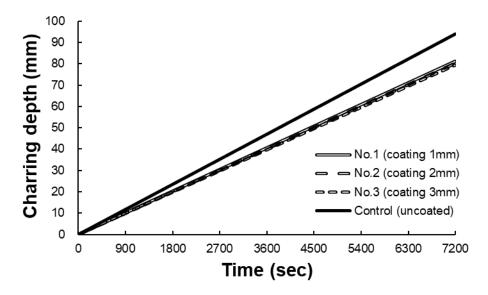
Fig. 15. Charring depth for required fire-resistance
