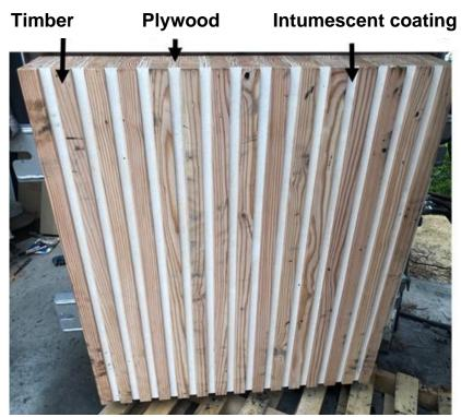
(a) Intumescent coated specimen (bottom of specimen)
