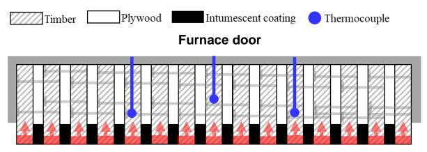
(a) One-dimensional heat transfer into timber (intumescent coated specimen)
