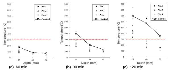
Fig. 10. Temperature at different depths depending on the time
