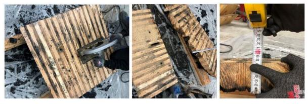
Fig. 13. Measurement of the residual depth of timber laminae
