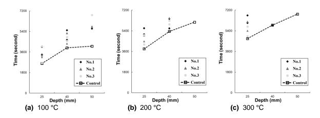
Fig. 12. Time when the temperature of each location reaches 100, 200, 300 °C
