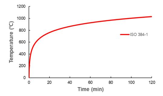
Fig. 7. Standard temperature-time curve in ISO 834-1(ISO 834-1:1999 1999)
