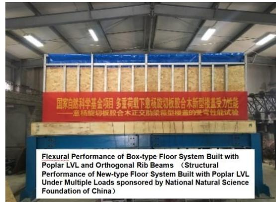
(b) Installed loading device
