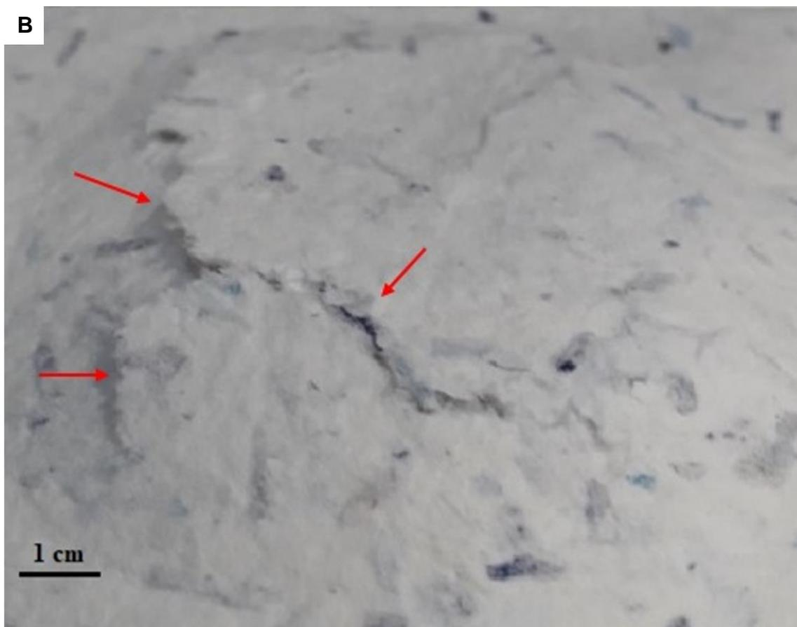
**Fig. 2.** A defect-free (A) and a damaged (B) molded pulp sample, defects in the damaged sample are highlighted with arrows
