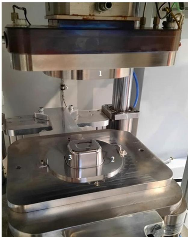
**Fig. 1.** Female mold (1), blank holder (2), and male mold (3) of MiniMold press-forming tool set
