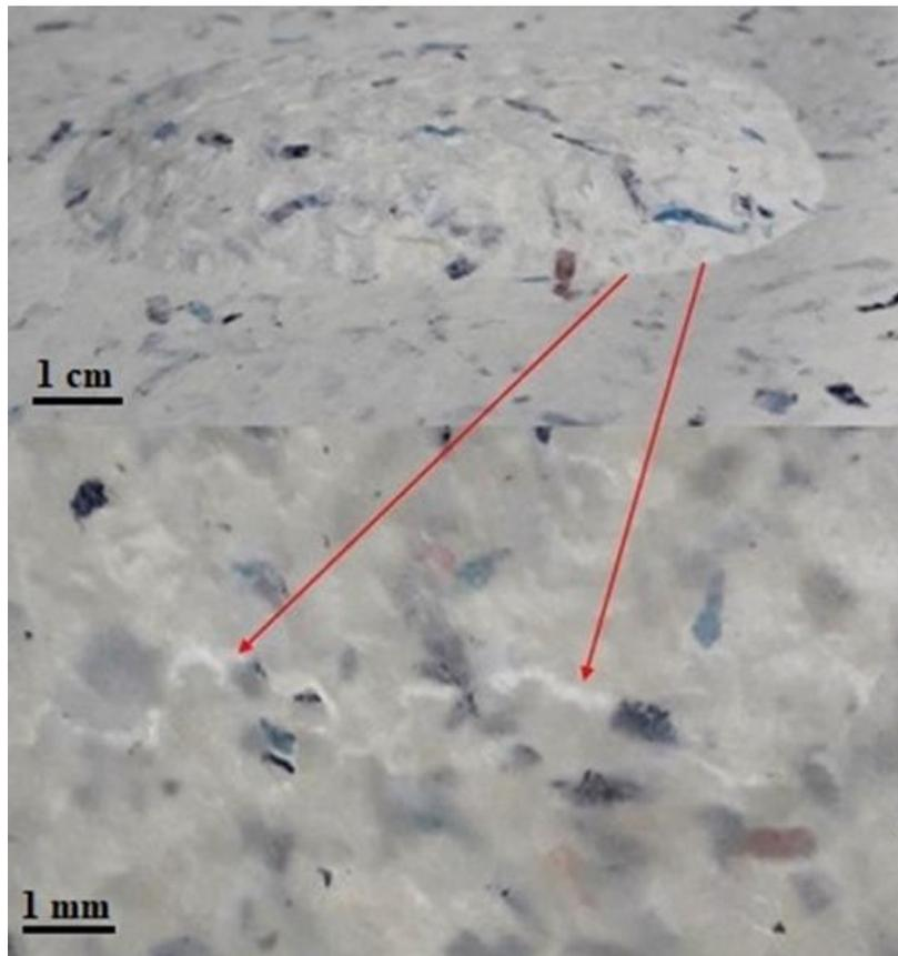
**Fig. 5.** Defects in flange region of a molded pulp sample (top), the defects are highlighted with arrows in an enlarged section (bottom) of the same sample
