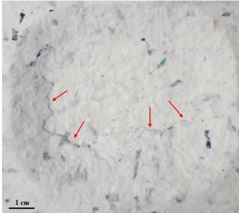
**Fig. 4.** Defects in bottom region of a molded pulp sample, the defects are highlighted with arrows
