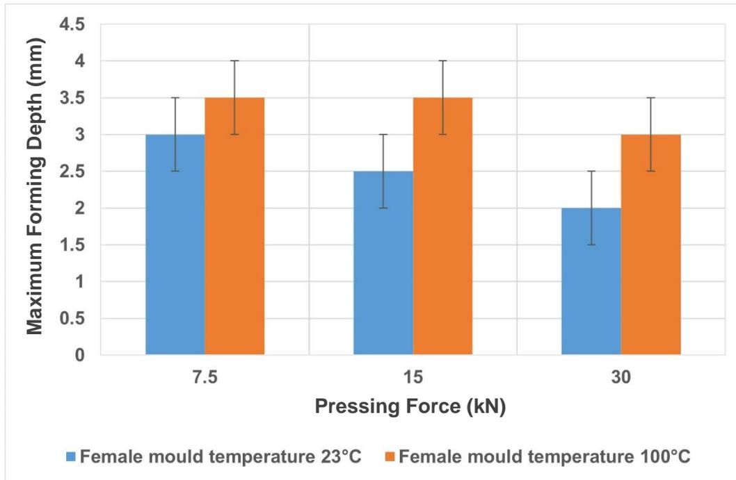
**Fig. 3.** Effect of female mold temperature and pressing force on maximum forming depth
