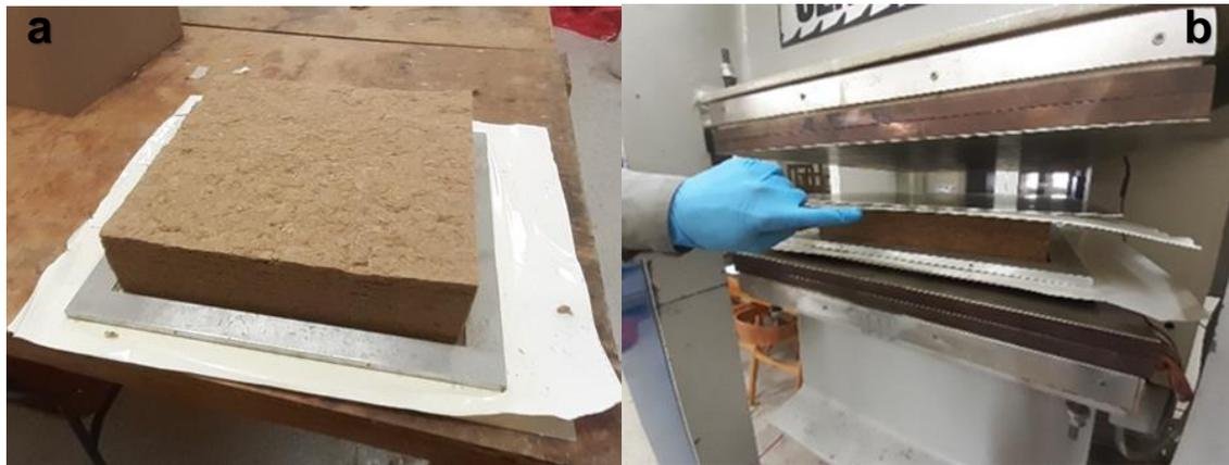
**Fig. 3.** a) Laying, pre-pressing b) Hot pressing of blended fibers in the mold
