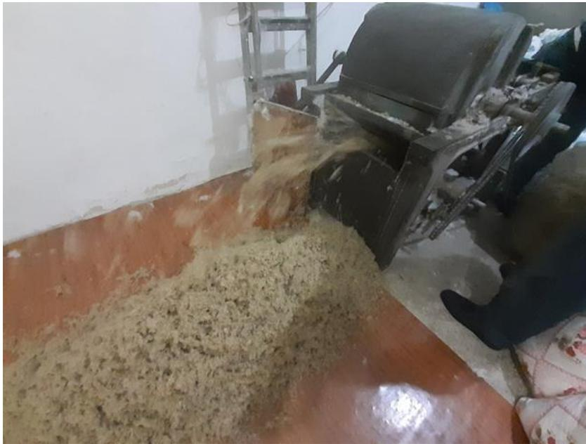
**Fig. 1.** Separation of stone wool into fibers in a wool carding machine
