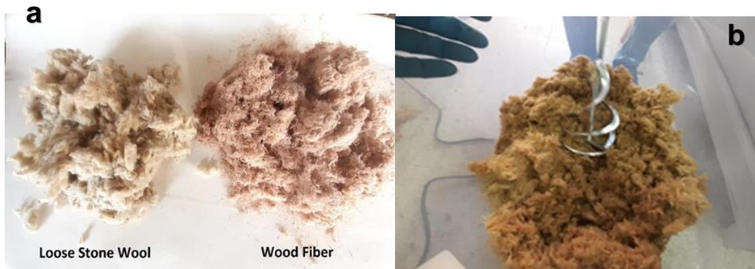
**Fig. 2. a)** The appearance of stone wool fiber and wood fiber **b)** Mixing of stone wool fiber and wood fiber
