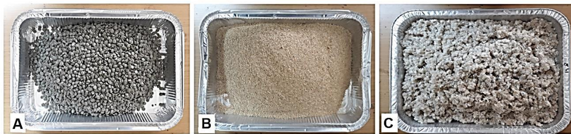
Fig. 1. Recycled polyethylene (A), pine wood flour (B), and ground Tetra Pak® box (C)
