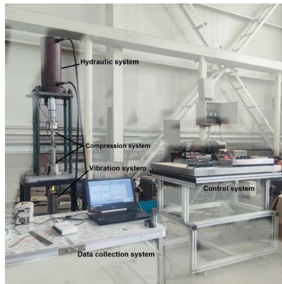
Fig. 3. The self-made biomass compressive test system
