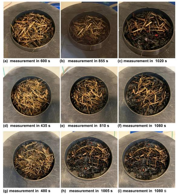
**Fig. 11.** Illustration of the combustion process at the critical temperature location. Key: specimen Hay 1 (a);(b);(c); specimen Hay 2 (d); (e); (f); specimen Hay 3 (g); (h); (i).
