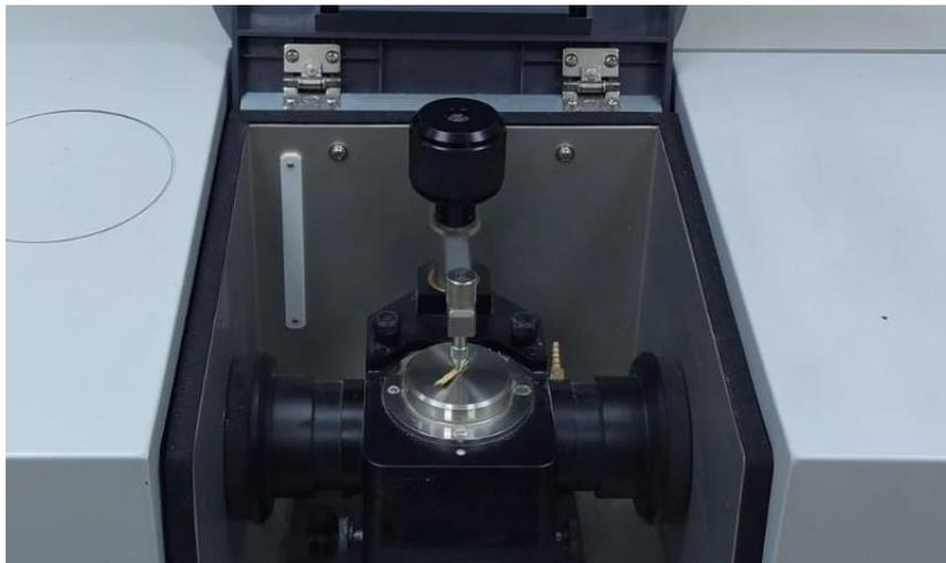
Fig. 1. The ATR Attached Shimadzu IR Prestige 21 spectrometer
