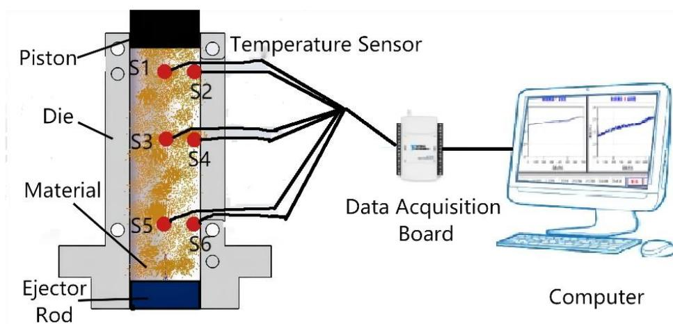
**Fig. 3.** Arrangement of the temperature sensors. S1, upper core; S2, upper edge; S3, middle core; S4, middle edge; S5, bottom core; S6, bottom edge temperature sensor
