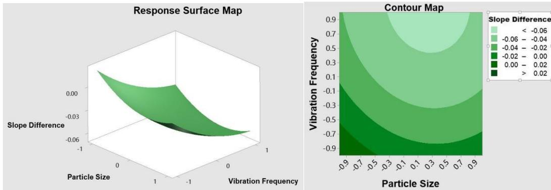
**Fig. 7.** Influence of vibration frequency and particle size on heat transfer at the upper of the die
