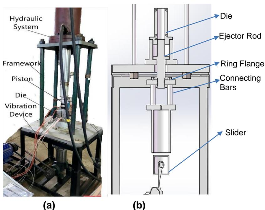
**Fig. 2.** (a) The experimental system; (b) the vibration device
