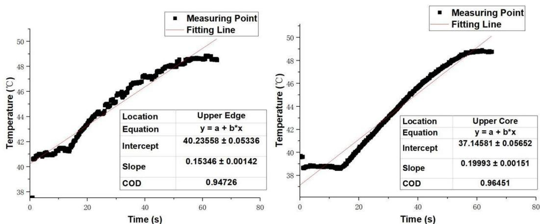
**Fig. 6.** Measuring point and fitting lines located in upper of the die under test order No.6 (Moisture content middle level, Vibration frequency high level, Particle size high level)
