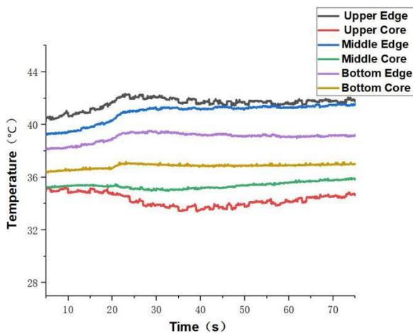
**Fig. 4.** Curve for the temperature without assisted-vibration compression (Moisture content middle level, Particle size high level)
