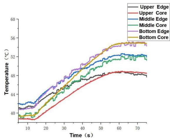
**Fig. 5.** Curve for the temperature with assisted-vibration compression (Moisture content middle level, Particle size high level)
