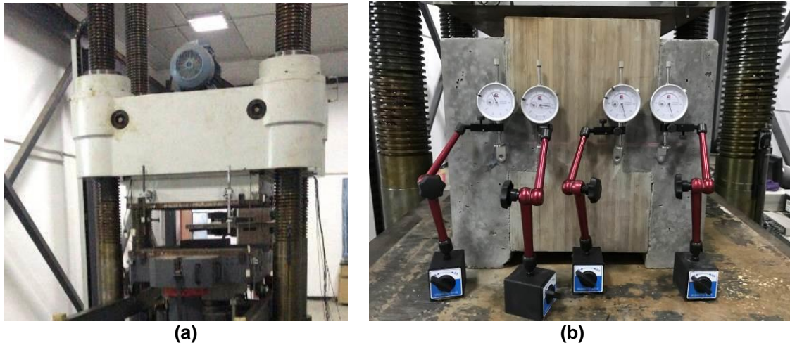
Fig. 3. (a) Microcomputer controlled electro-hydraulic servo shear testing machine; (b) Arrangement of dial indicators
