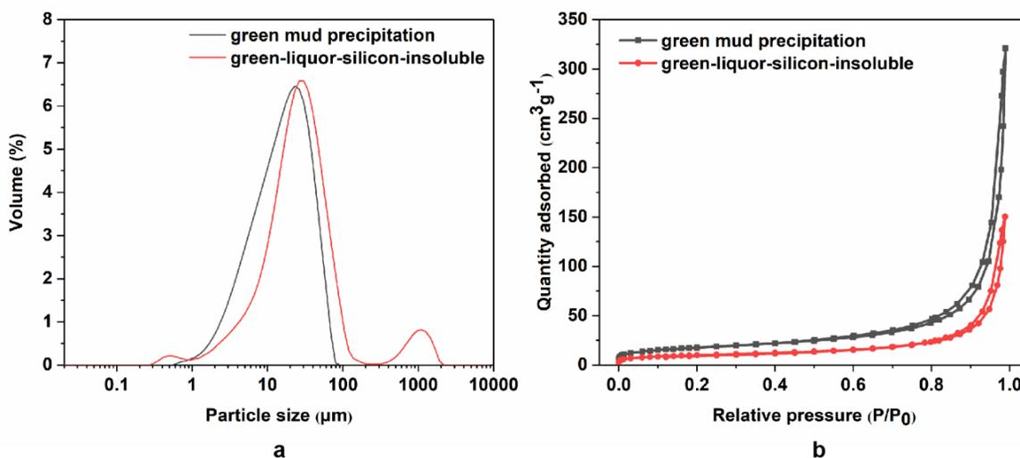
**Fig. 6.** Analysis of green mud precipitate and the GLSI substance: a: particle size; and b: BET surface area
