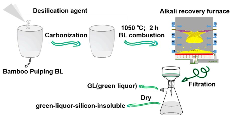
**Fig. 1.** Schematic of green liquor desilication *via* black liquor combustion
