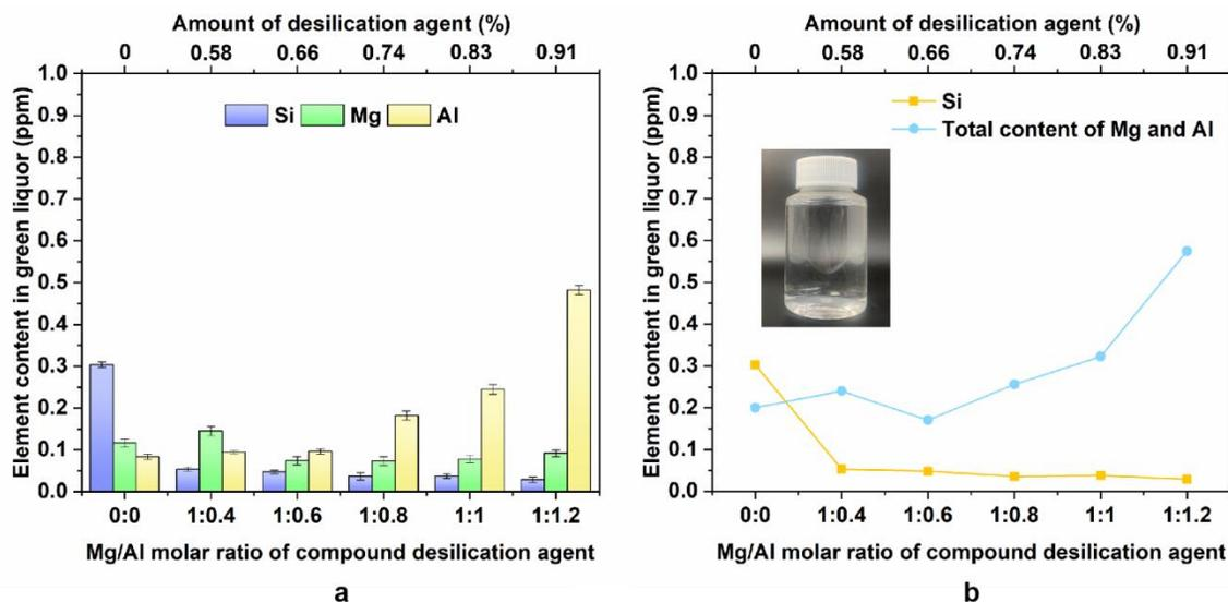
**Fig. 3.** Mg-Al compound as desilication agent: a: elemental content in GL; and b: content of residual desilication agent in GL
