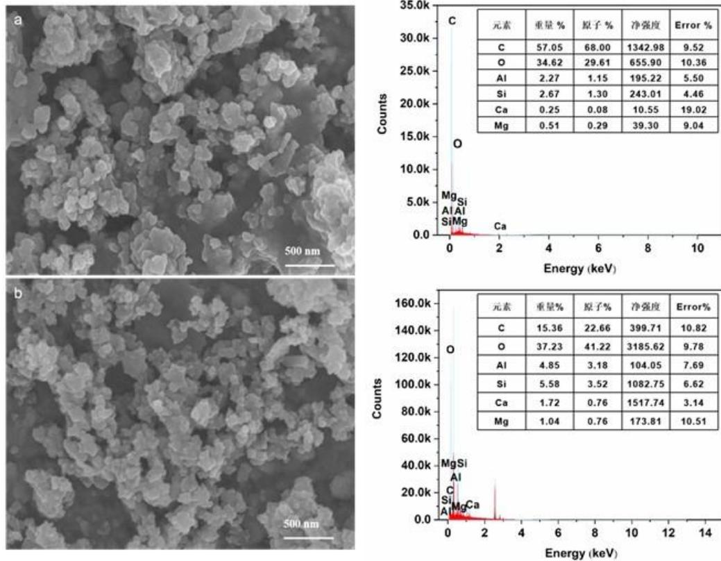
Fig. 4. SEM images and EDS results: a: green mud precipitate; and b: GLSI substance
