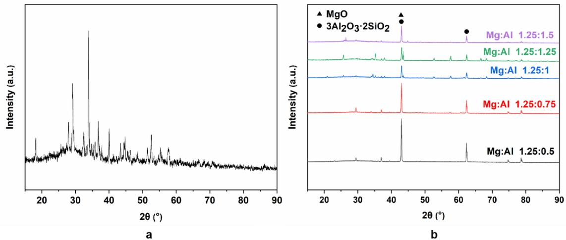
Fig. 5. X-ray diffraction patterns: a: green mud precipitate; and b: GLSI substance
