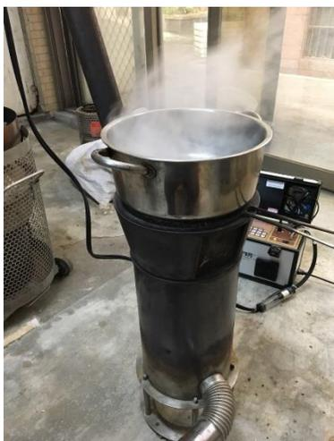
**Fig. 2.** Diagram of the custom-made boiler
