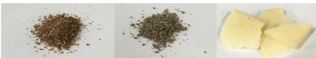
Fig. 1. Sample of wooden material (wood), wood mixed with PU, and rigid PU foam
