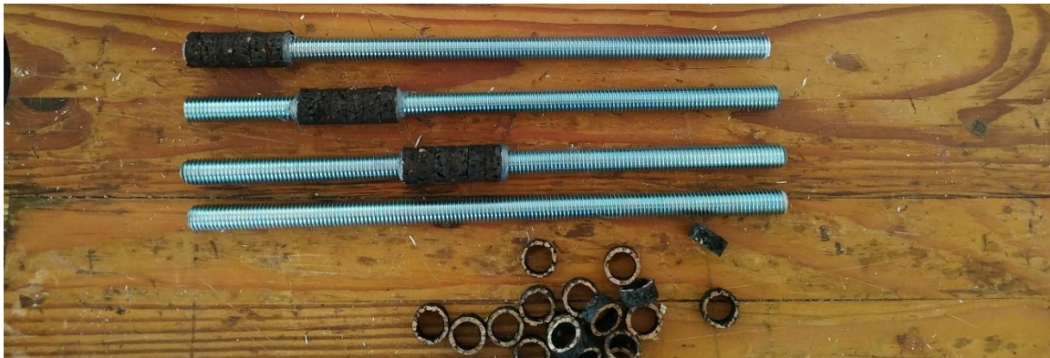
Fig. 2. Cork washers fixed of the rods for each sample population shortly before being embedded in samples: R – reference (no defects), T, M, B – glue-free zones in top, middle, and bottom parts of the embedded rod, respectively
