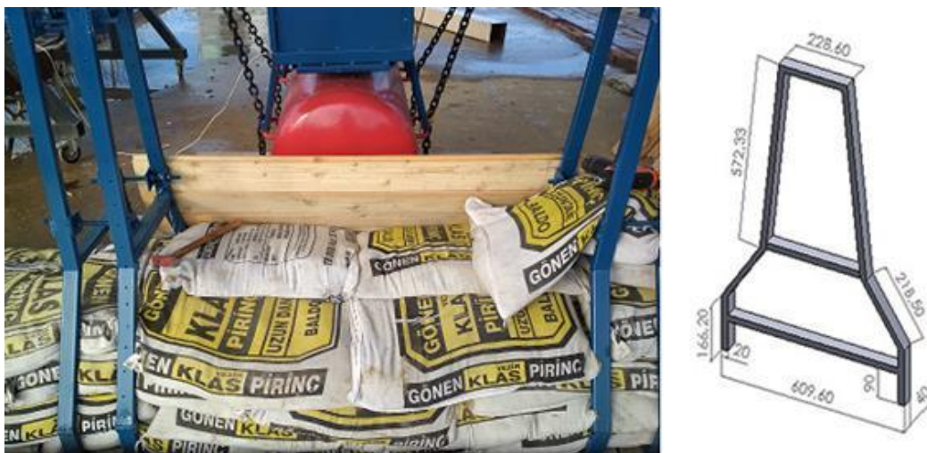
Fig. 2. Steel frame and the dimensions; all units are in mm
