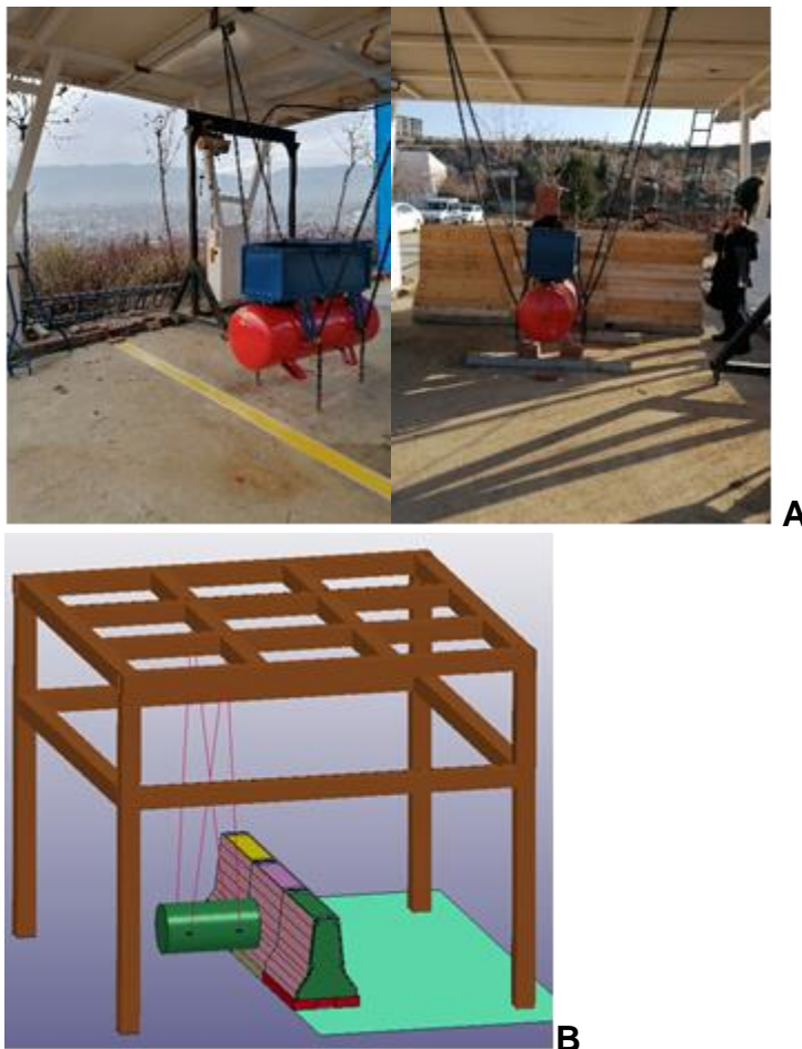
Fig. 7. (A) Pendulum system and (B) its FE model
