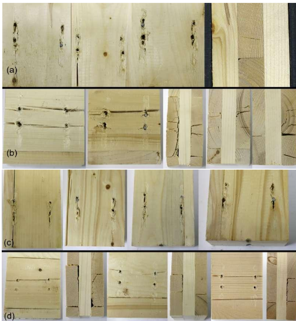
Fig. 8. Typical failure appearances of the screw connection CLT specimens during the shear tests: (a) type 5; (b) type 6; (c) type 7; and (d) type 8
