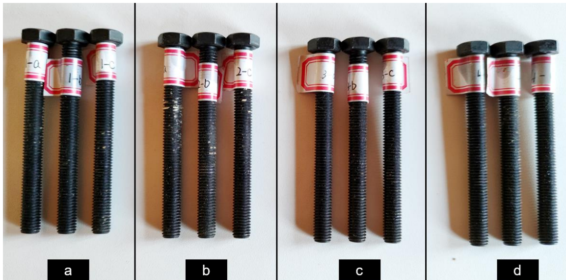
Fig. 5. Deformation of the bolts after the test: (a) bolts of type 1 specimens, (b) bolts of type 2 specimens, (c) bolts of type 3 specimens, and (d) bolts of type 4 specimens
