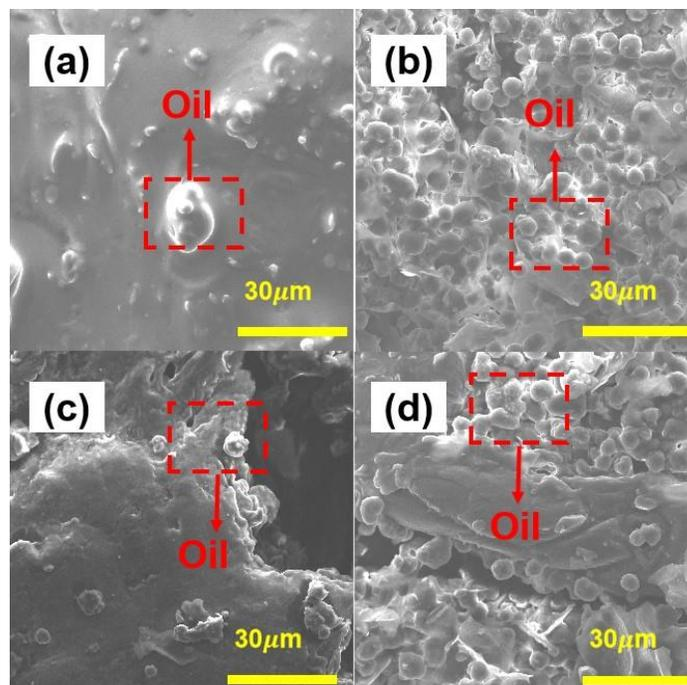
**Fig. 10.** SEM images of walnut before and after extraction: (a) Walnut; (b) After Soxhlet; (c) After pressing; and (d) After ultrasonic
