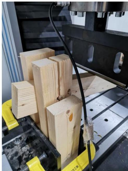
**Fig. 5.** Testing setup using the WDW-300E universal testing machine
