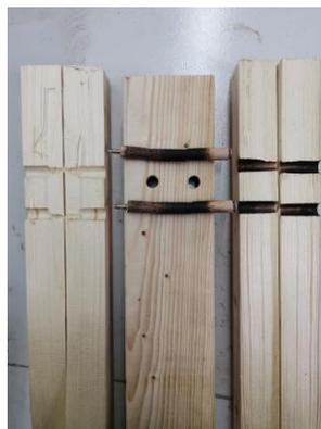
**Fig. 7.** Failure mode of composite dowels
