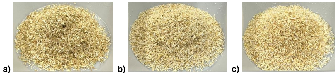
Fig. 1. Biomass was sieved to a particle size of 0.6 to 1.18 mm including: a) intermediate wheatgrass grown at the Froid location, b) canola grown at the Froid location, and c) canola grown at the Ras location.
