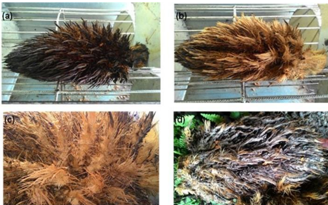
Fig. 3. Physical effect of OPEFB bunch for (a) untreated OPEFB, (b) HPWSS treated OPEFB, (c) closed-up of HPWSS treated OPEFB, and (d) fungal growth on HPWSS treated OPEFB after 3 days
